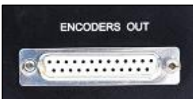
08.37 Encoder out connector from the cranes.
