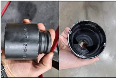
02.06b Socket KM tool with 2 teeth cut.
