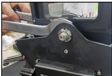
06.05 Adjusting the eccentric axis.
