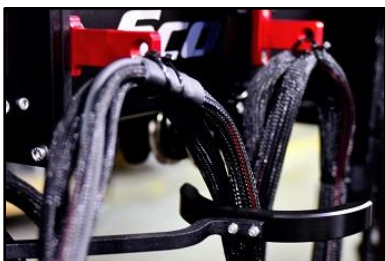
02.37 Cable holders and cable diverter.
