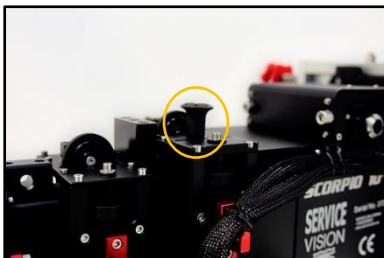
02.22 Telescopic sections locking pin.
