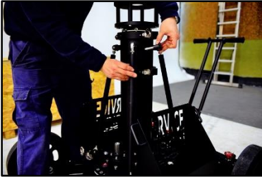
10.11 Tensors on the column.
