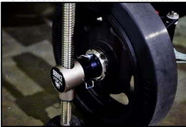
02.07 Leveling Jack attached.
