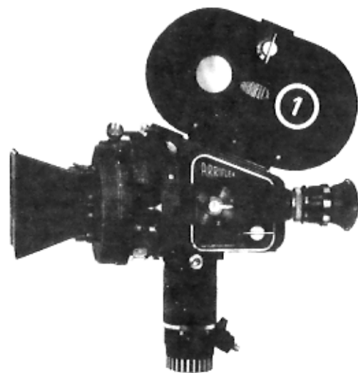
Fig. 1: A sunshade belongs to the standard equipment of the ARRIFLEX 35 II C. Either this or the practical adjustable sunshade with bellows (available as a special accessory under Cat. No. 2001) should be used for all shots in order to achieve maximum sharpness and contrast.
