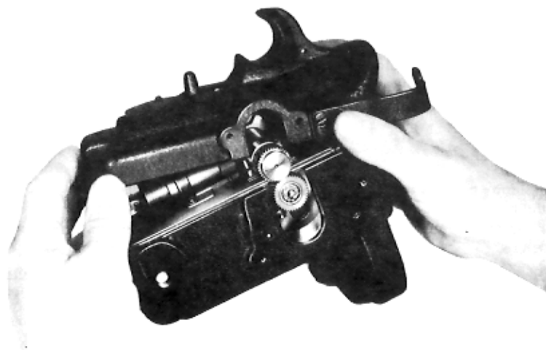
Fig. 18: After lifting the gear cover so that it slides over the driving shaft, tilt it forwards at a 45° angle towards the shutter bulge and lift it off.
