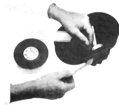
Fig. 4: The film is passed through the feed sprocket parallel to the wall until it emerges through the left-hand channel.
